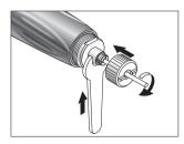
Insert the chuck key up to the limit stop in the chuck and screw clockwise.Hold the shaft firmly with the spanner.
