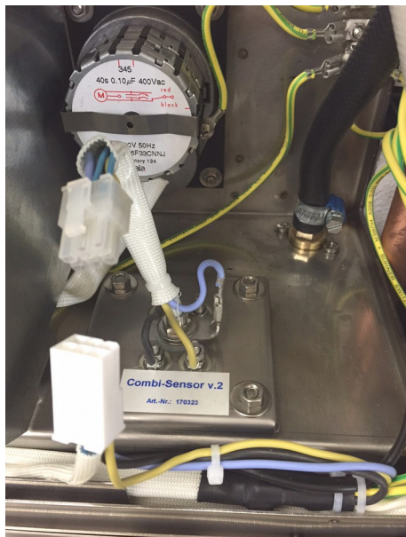
Pull off the sensor plug (6-pin)
