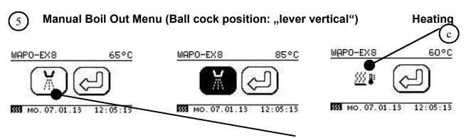
The manual boil out process is initiated by touching the **boil out symbol**.
