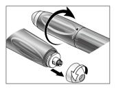
• Turn the front sheath clockwise up to the limit stop. Unscrew the tip anti-clockwise.
