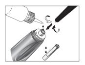
• Clean the inside and outside of the shaft using the cleaning brush. Apply 2 drops of oil into the hole in the shaft and outside of the chuck.
