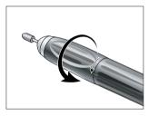
2 Turn the front sheath anticlockwise until it engages audibly.
