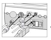
Connect the motor cable, operating controls, footoperated starter, air hose (HSM-50) and mains cable.
