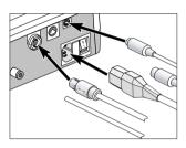
• Connect the motor cable, operating controls (optional), air hose (HSM-50) and mains cable.
