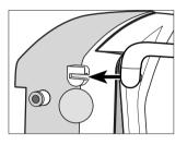
• Push in the fitting for the blow out function up to the limit stop. (HSM-50).
