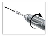
Turn the front sheath clockwise up to the limit stop. Push in the rotary tool up to the limit stop or remove.
