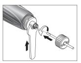
② Insert the chuck key up to the limit stop in the chuck and unscrew anticlockwise. Hold the shaft firmly with the spanner.
