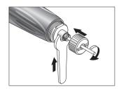
**6** Insert the chuck key up to the limit stop in the chuck and screw clockwise. Hold the shaft firmly with the spanner.
