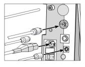
2 Connect the motor cable, operating controls, footoperated starter (optional), air hose (HSM-50) and mains cable.
