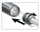
Assemble and tighten the cap.
