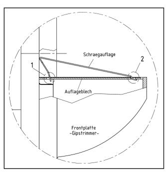
Make sure that items 1 and 2 are inserted correctly in the support plate.
