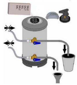
Regeneration mode (valve "C" to the left, valve "D" to the right)
