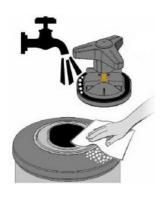
Check the seal on the lid and the top part of the Wasi-Clean for any residues of salt or resin, clean if necessary and then fit the lid and screw it tight.
