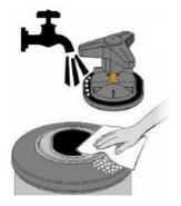
Check the seal on the lid and the top part of the Wasi-Clean for any residues of salt or resin, clean if necessary and then fit the lid and screw it tight.
