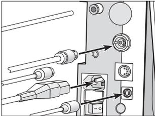
**2** Connect the motor cable, operating controls, foot-operated starter (optional), air hose (HSM-50) and mains cable.
