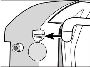
**1** Push in the fitting for the blow out function up to the limit stop. (HSM-50).
