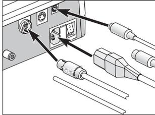
**1** Connect the motor cable, operating controls (optional), air hose (HSM-50) and mains cable.
