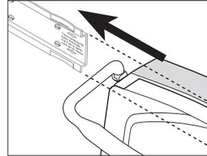
**3** Insert control unit up to the limit stop on the holding plate.
