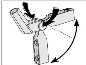
❷ The support can be moved into a variety of assembly positions by simultaneously pressing both buttons on the joint.
