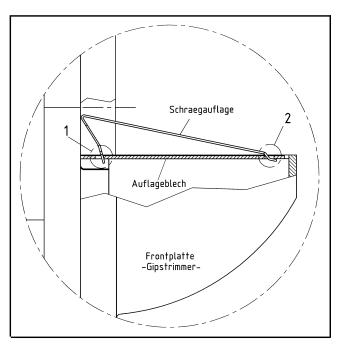
When installing the angled mount, ensure that positions 1 and 2 are correctly located on the base.
