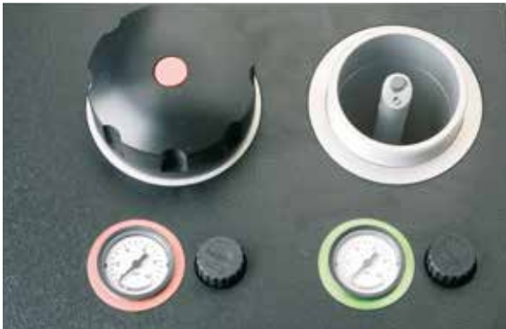
Individual blasting pressure for each chamber, 1-6 bar
