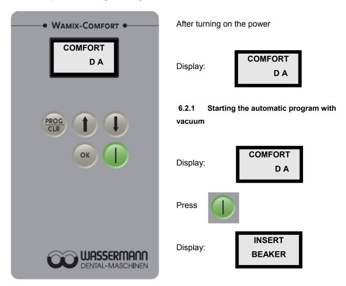
To start the program, insert the beaker in the flange from below. Hold the beaker until mixing starts.
