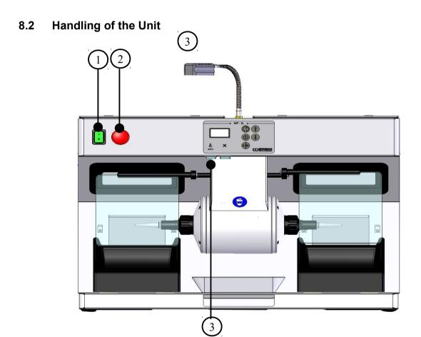
The WP-3000 Ex II is turned on with the main switch. The motor speed is controlled using the arrow keys. The extraction and the LED spot can be manually turned on and off.
