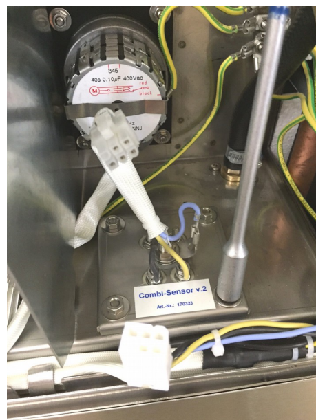
(4x M5) unscrew the nuts
